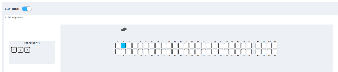
FIGURE 19 Displaying LLDP Neighbor Devices
